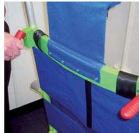
9. When in position, open the two red spring clips. This will allow the handle to be raised. Once raised, close the two red spring clips and ensure they have re-engaged, this will lock the handle in place.
