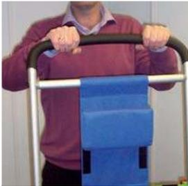
10. Transfer hands from pushing position on the sides, to the top of the handle. Place your foot on the green track assembly bar and lever the chair back.
