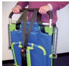
17. Pass the lower part of the support harness through the foot rest and connect to upper harness. Place chair back into storage location and replace protective cover.
