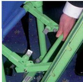
8. Pull the track back and pull the crossbar towards/upwards to you and close the spring clips. Ensure they have re-engaged by pushing down on the track unit.
