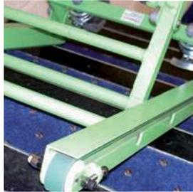
11. Keeping the tracks firmly in contact with the stairs, ensure a firm grip, apply downwards pressure on the handle and allow the chair to operate downwards.
