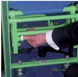
7. Pull open the two spring clips located at the back of the chair between the tracks.
