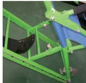
9. Once the chair is at the stairwell, any bumps, strips or stair protectors can be traversed by putting your foot on the bar as shown.
