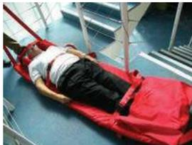
8. Once on the stair landing, lower the Evacuslider into the static position and prepare for next flight of stairs.
