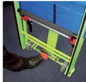
14. Ensure the brake mechanism is locked.
