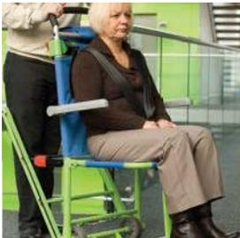
13. Once you reach a landing, return the chair to four wheels and manoeuvre to the next flight of stairs. When you get to the ground floor manoeuvre to final exit.
