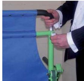
3. Undo the spring clips on the handle, lower, close clips and lift to lock.
