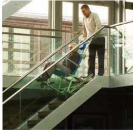
11. Manoeuvre the chair forward onto the top two steps, make sure the tracks stay in full contact with the stairs.
